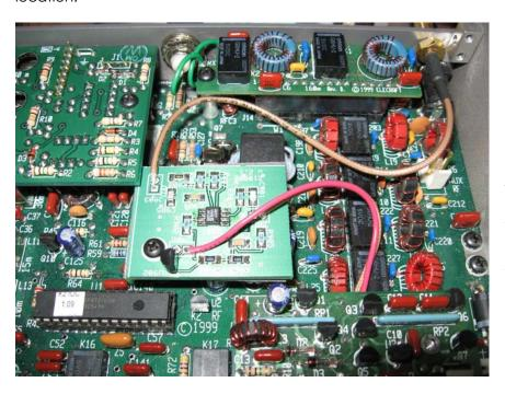
Bob's K2 with the buffer amplifier in place. Note the SMA connector mounting in the space between the 160 meter board and the edge of the back panel. The SMA bulkhead connector is supplied with one lockwasher intended to be used on the outside of the enclosure, between the nut and panel. Bob suggests using a second internal tooth lockwasher on the inside. If you follow this suggestion, a 1/4" (6mm) internal tooth lockwasher can be obtained at any hardware store.
