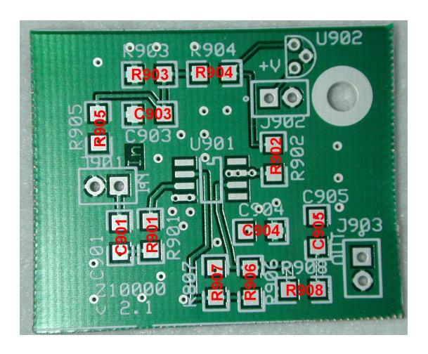
The photograph shows an earlier version of the PCB. Later PCBs correct the silk screen error identifying R907 as R807, and slightly rearrange other silk screen legends. In addition, production circuit boards may be slightly smaller than in the photographs.
