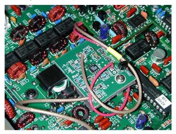
Now that you know where the buffer amplifier will be located, determine where the output SMA connector will be installed.
