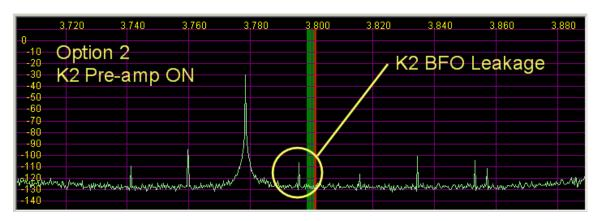
The images show a significant reduction in BFO leakage, on the order of 30 dB.
